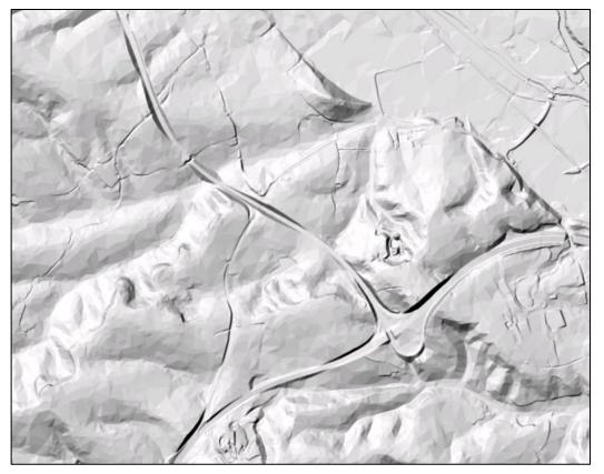
In the above image the OS Terrain 5 grid has been shaded in a GIS.
