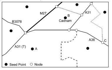
Lines and points from the geometric structure become features when a meaning, the feature code, has been added – for example, roads are created from lines, or settlements from points.
