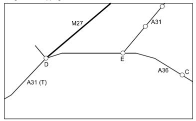
Figure 2.4c: Separate storage of overlapping features
