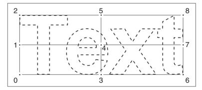
Names are normally placed on the printed map parallel to the horizontal grid. However, names of linear features are orientated to appear parallel to them, for example, rivers.
