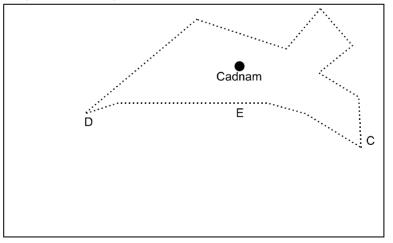
The common line (D–E) to the A31(T) and the settlement polygon, and the common line (EC) to the A36 and the settlement polygon, each represent two lines. The geometry of each feature is stored separately in the data.
