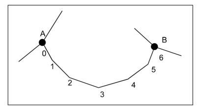
Points A and B are nodes, as they intersect with other features. The line A–B is the link and, in this example, is made up of six individual line segments.
