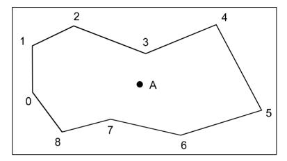
Point A is the polygon seed point for the area; attached to this point will be attributes such as the feature code, which defines it, and its definitive name – if it is named on the map. The polygon in this example comprises nine individual line segments.
