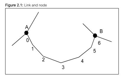
Points A and B are nodes, as they intersect with other features. The line A–B is the link and, in this example, is made up of six individual line segments.
