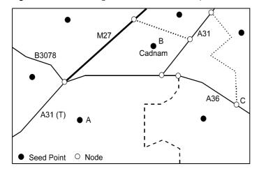
Lines and points from the geometric structure become features when a meaning, the feature code, has been added – for example, roads are created from lines, or settlements from points.
