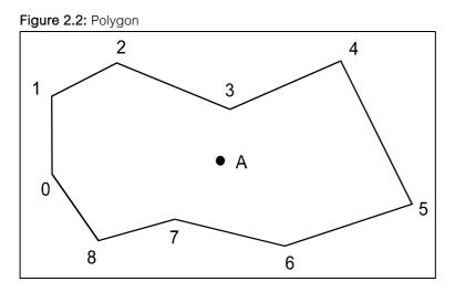
Point A is the polygon seed point for the area; attached to this point will be attributes, such as the feature code, which define it, and its definitive name – if it is named on the map. The polygon in this example comprises nine individual line segments.
