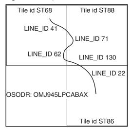
Unique identifiers have been assigned to all existing roads (links and nodes), railway links and railway stations and to seed points for administrative areas, DLUAs, hydrology (inland water) and woodlands. Any of these features that are new to Meridian 2 after the initial allocation will be assigned an appropriate unique identifier when the database is refreshed.
