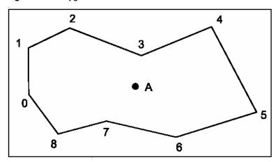
Point A is the polygon seed point for the area: attached to this point are attributes such as the feature code, which defines the polygon and its definitive name. These attributes may be transferred to the polygon itself. The polygon in this example comprises nine individual line segments.
