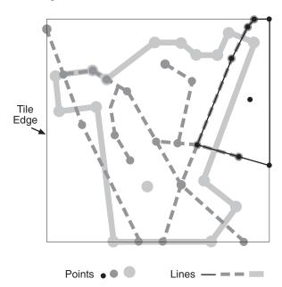
Points and lines from the geometric structure become features when an attribute, the feature code, has been added, for example, DLUA seed points are created from points, or DLUA boundaries from lines.
