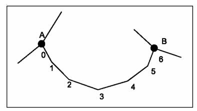
Points A and B are nodes, as they intersect with other features. The line A–B is the link, and, in this example, is made up of six individual line segments.
