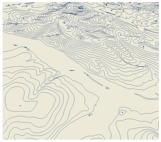
OS Terrain 50 contours and spot heights displayed as a heighted raster in a GIS.
